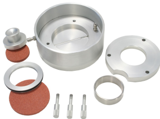
Consolidation cell exploded view
